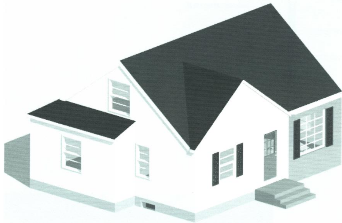
An axonometric of the master bedroom addition shows the low shed roof tucking in right under the attic window.
